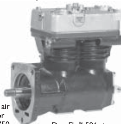
DuraFlo™ 596 air compressor or BA-922™ air compressor (exterior view is very similar)
